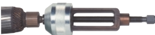
Removing an inner ball bearing race with the aid of a pulling chuck type 23.
