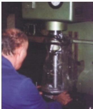
A hydraulic shop press set up with a T-UFP-2 protective blanket. The blanket fully encloses the work, and the work progress can be observed and controlled from start to finish.
